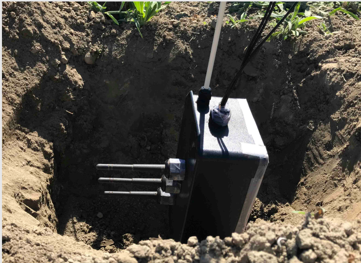
Waterproof box holding the RX antenna array
